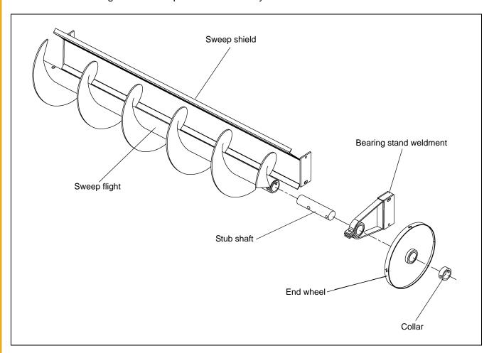
Figure 3L End Wheel Assembly
